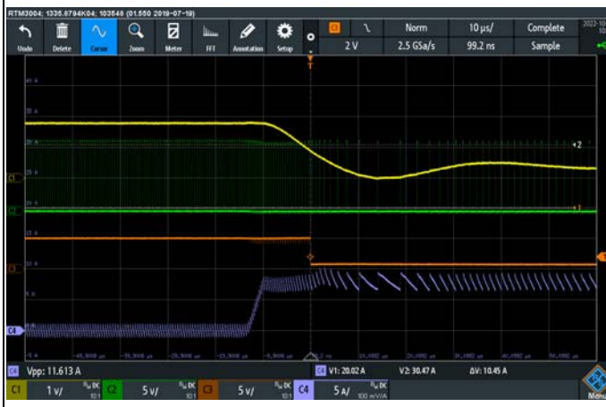
Figure 23 SCP for REG_CYC_OCP [1:0] =2 CH1: VOUT CH2: SW CH3: PG CH4: IL
