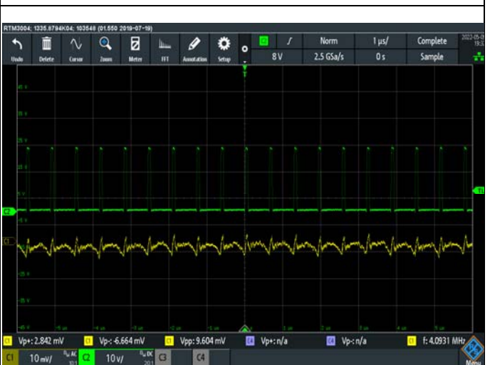
Figure 20 VOUT Ripple and SW 6A CH1: VOUT CH2: SW
