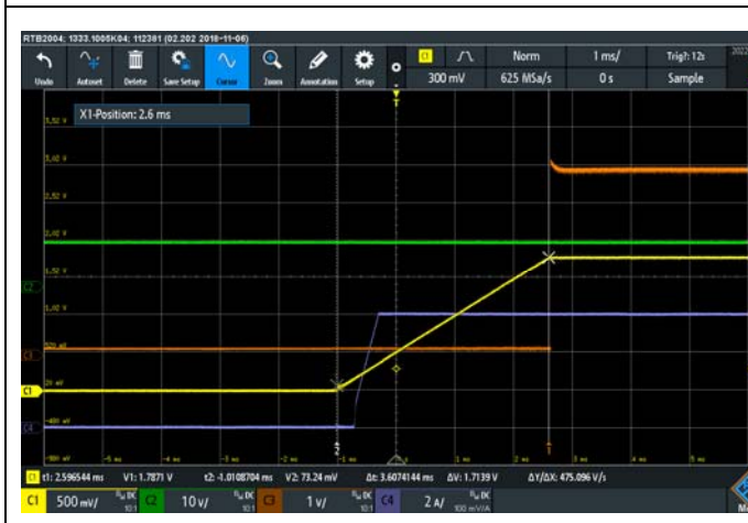
Figure 17 Power on for EN and Soft-Start CH1: VOUT CH2: VIN CH3: PG CH4: IOUT
