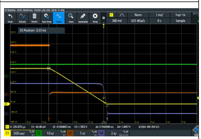
Figure 18 Power off for EN and Soft-off CH1: VOUT CH2: VIN CH3: PG CH4: IOUT
