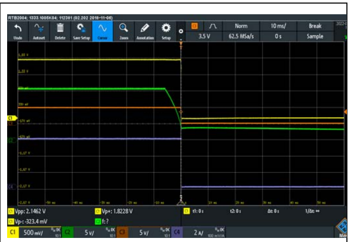
Figure 16 Power off for PVIN CH1: VOUT CH2: VIN CH3: PG CH4: IOUT
