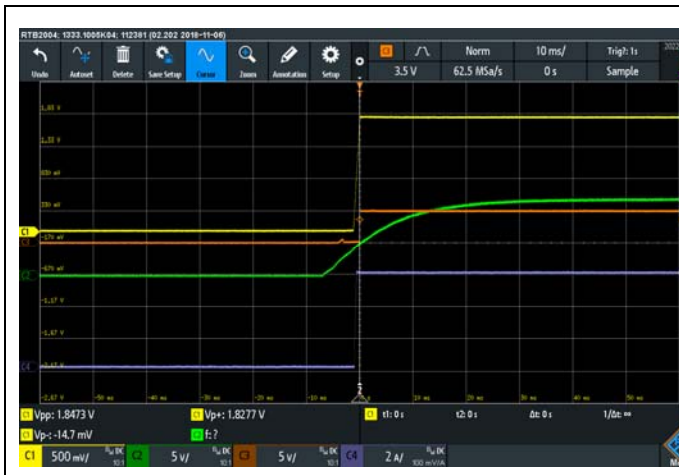
Figure 15 Power on for PVIN CH1: VOUT CH2: VIN CH3: PG CH4: IOUT
