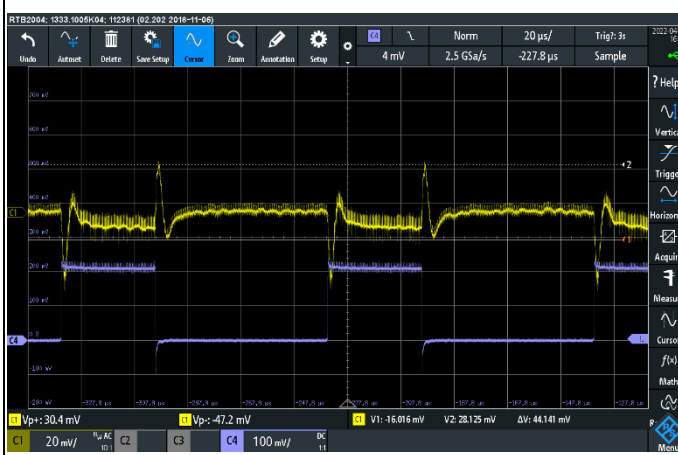
Figure 25 Load Transient 10KHz Load Range=0~4.2A Slew rate 7.5A/μs CH1: VOUT CH4: IOUT
